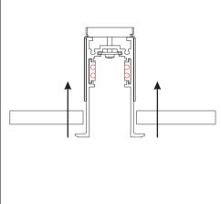
**step 4.:** Screw the fixation parts in order to open the tool.
